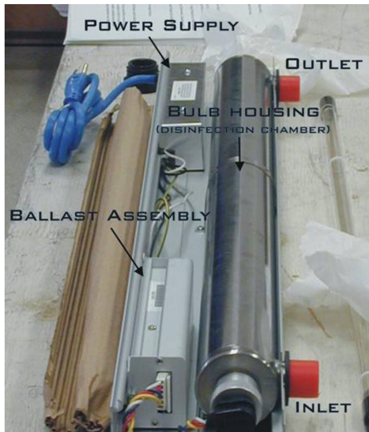
Figure 5: Basic components of UV system
